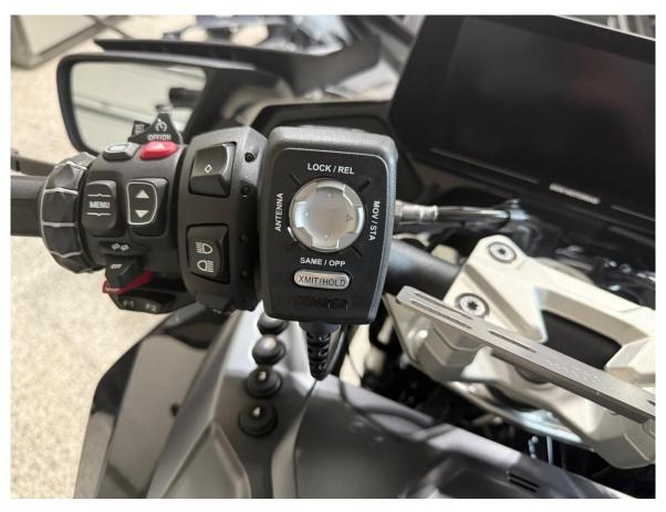
All of the various mounts for radar remotes, microphones and phone attach to the casting which also mounts the authority switch cluster. To remove the plugs, tap a small slotted screwdriver into the plug and unscrew it. Trying to pry the plug out usually ends in disaster! As the threaded holes are blind, do it right by unscrewing it as shown at right.
